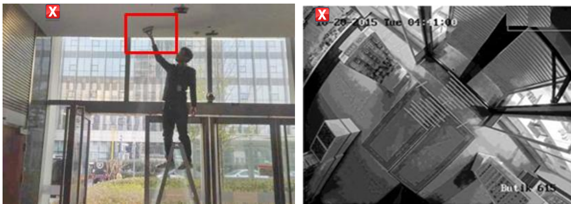
Figure 3-8 Passenger Flow in Horizontal Direction (Wrong)
